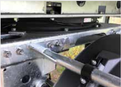
Axle seat Hot-dip galvanised
