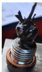
Fig. 27: Check metal flakes at drain plug
