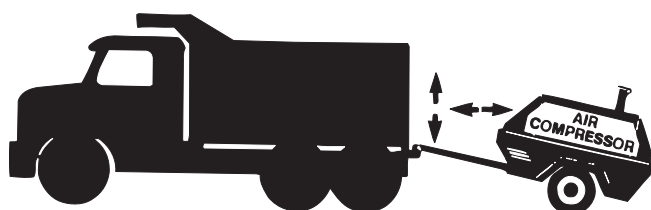
Improper Mounting Height (causing excessive vertical and horizontal movement)
